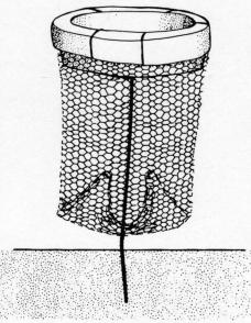
Like a crabpot on a stick, this chicken wire trap catches crawfish. The trap stands on its rod above the bottom of the pond and attracts crawfish with various kinds of bait. The crawfish enter through wire cones at the bottom and, like crabs, find it impossible to exit because of their stiff shells.
