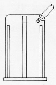
One way to mass produce crawfish traps is to build a wooden jig. Use the jig to form the chicken wire, then make good use of a soft drink bottle to mold two coneshaped entry points for the crawfish.
